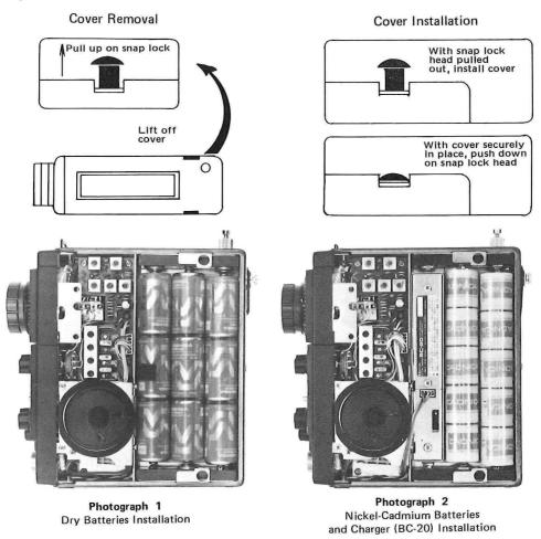
Nickel-Cadmium Batteries and Charger: BC-20
